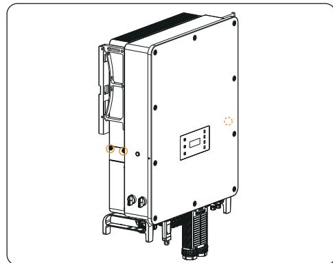
Figure 11-12 Dismantling screws
