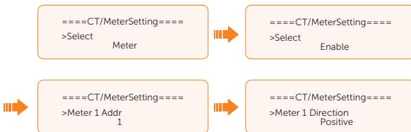
Figure 14-16 Setting meter for the inverter
