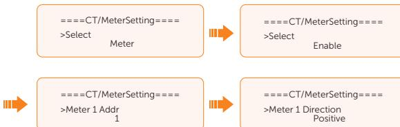
Figure 14-21 Setting meter for the inverter
